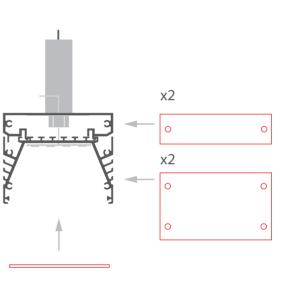
5. Install the W-KG-Z ceiling fasteners. The fastener installation manual can be downloaded at www.klusdesign.eu. Connect the cables, each for the single power pole to the fasteners. The cables should go through a pre-drilled hole just under the masking cover of the fastener.
