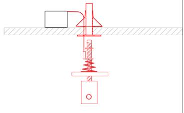
6. Mount the fixture with rods into the ceiling fasteners. Connect the cable to the power supplier, leading it through a pre-drilled hole in the ceiling.
