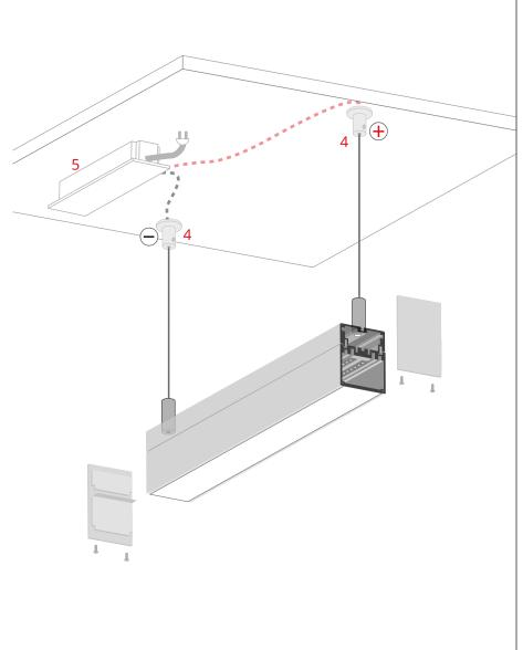
Suspend the lighting fixture from the ceiling fasteners (4) which are connected to the power supply (12 V / 24 V) (5).
