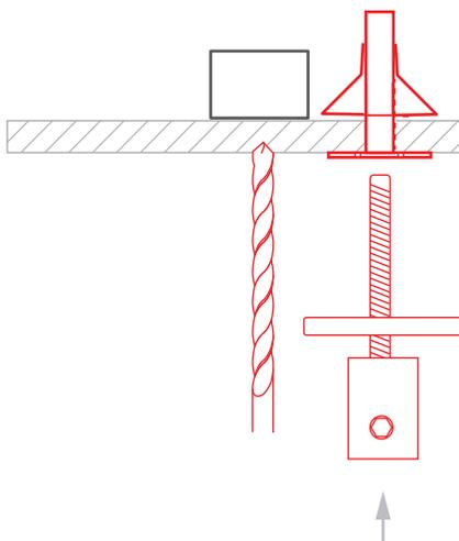
**6.** Mount the fixture with rods into the ceiling fasteners. Connect the powering cable.
