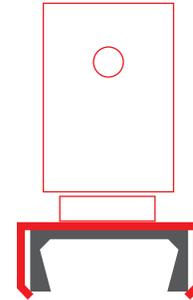
**3.** Mount the LED strip in the extrusion and lead the cable through a pre-drilled hole.
