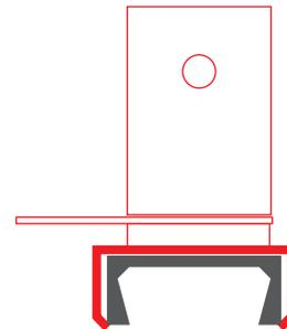
**3.** Mount the LED strip in the extrusion and lead the cables through pre-drilled smaller holes. Then lead them to the connectors of the DP-MOC-ZZ fasteners. Each hole should lead a cable with one power pole, LED strip has to be cut before installation, so the wires can be easily routed to the holes.
