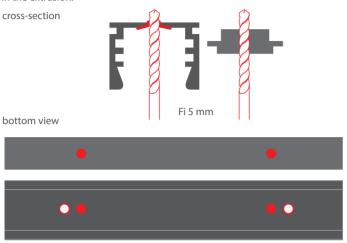
**3.** Mount the LED strip with the insert in the extrusion and lead the cables through pre-drilled holes in the insert and the extrusion. Then lead them to the connector sof the DP-ZZ fasteners. Each hole should lead a cable with one power pole, LED strip has to be cut before installation, so the wires can be easily routed to the holes.
