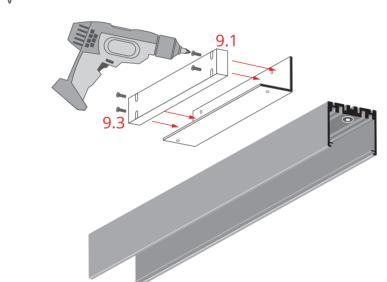
Mount the power supply (12 V / 24 V) (9.1) to the insert with bolts (9.3).
