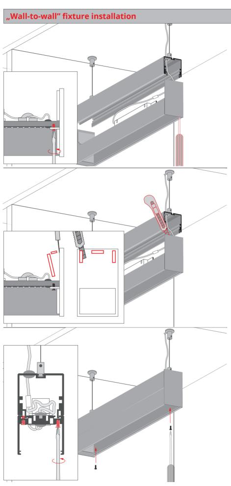
In case of "wall-to-wall" installation it is necessary to mount the fixture with the end caps from the bottom.
