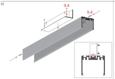
Attach the insert to the profile with the connector (9.4).
