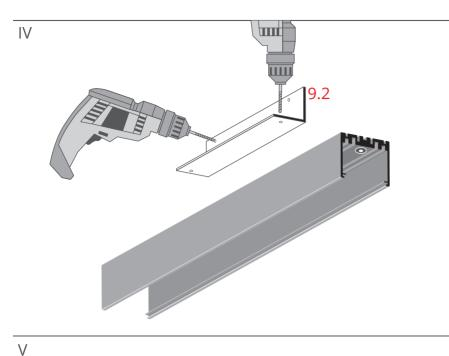
Drill the holes for bolts and connectors in the insert (9.2).
