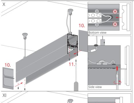
Insert the end cap bolts (11) in threaded channels (as shown in the figure).
