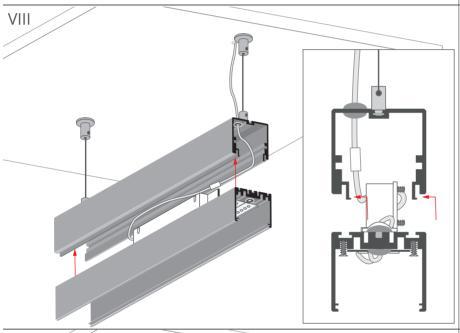
Connect the power cables. They can be placed in the chamber inside the mounting strip.
